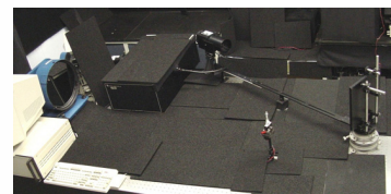
During actual use, the FEL lamp is housed inside an enclosure to block stray light.
